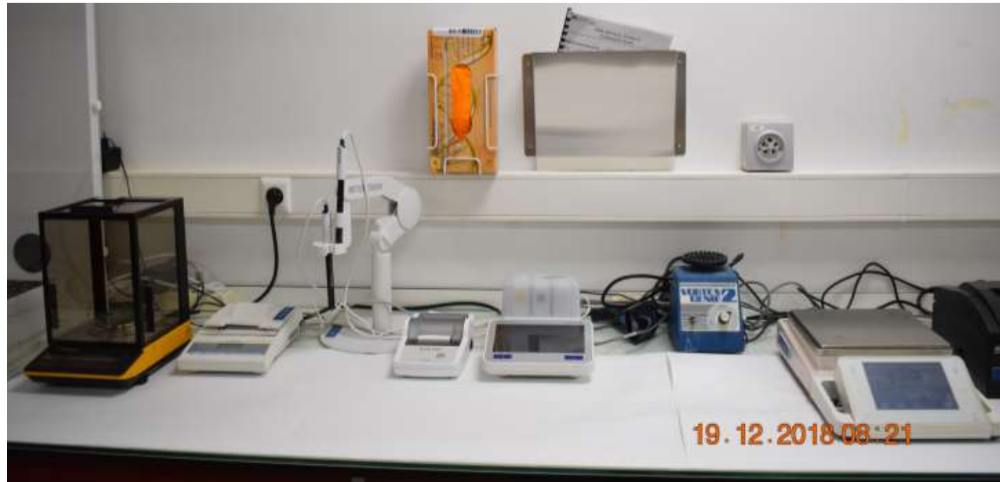
Balances and SevenExcellence multimeter (pH-Conductivity-Sodium)
